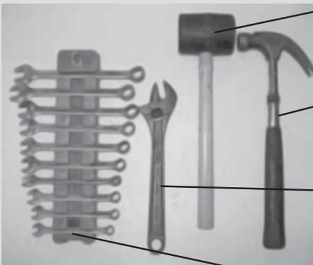
Rubber mallets are useful for careful tapping of moulds to help with demoulding.
