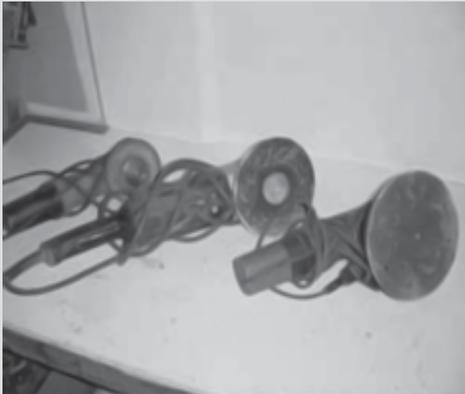
Electric disc grinders are mainly used for sanding away damaged FRP, but also for abrading the laminate prior to assembly and to improve secondary bonding. They can be fitted with rubber backing discs for use with 40-grit sandpaper.
