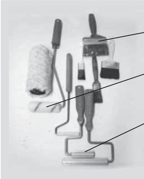
The brushes are used for applying gel coat, and can also be used for getting polyester resin into tight corners and onto small details.
