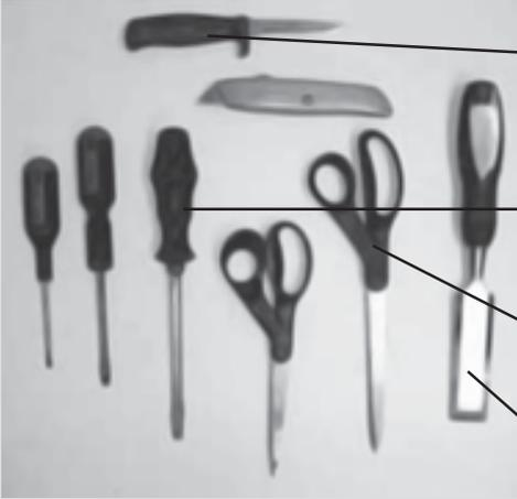
A regular knife or utility-type knife with extra blades can be used for cutting dry reinforcement (CSM) or "soft" laminate from edges.
