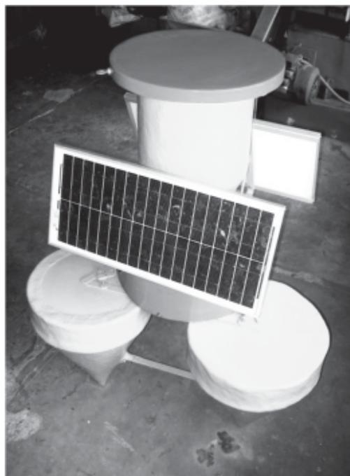
View of automatic fish feeder powered by solar panel
