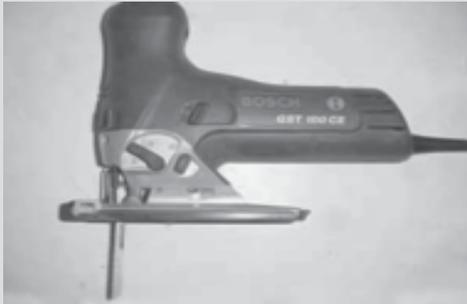
A power saw with a laminated hard metal blade, like the one shown here, is useful for cutting both wood and FRP laminate.
