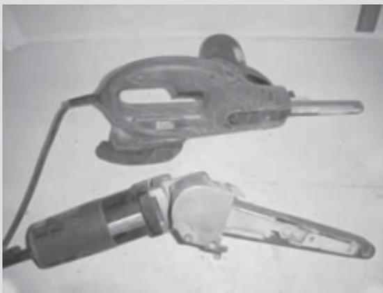
Belt sanders are excellent for sanding in preparation for repairs and for getting into tight corners.
